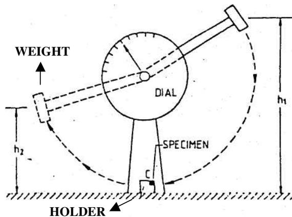
**Figure 1.** Schematic of a conventional Pendulum Impact Tester
