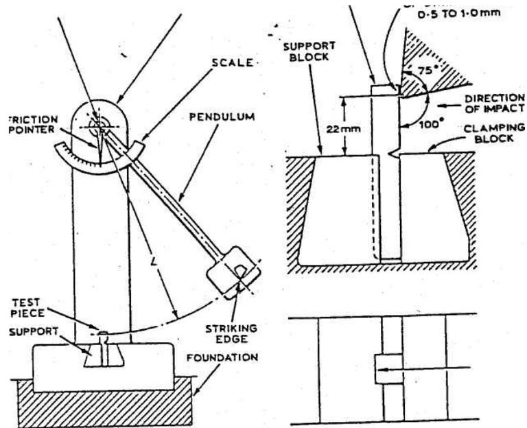
**Figure 2.** Basic Principle of Izod Impact Test
