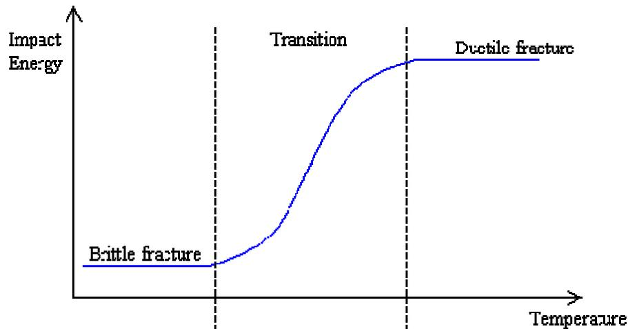
Figure 3: Schematic Presentation of the Ductile-to-Brittle Transition Curve.
